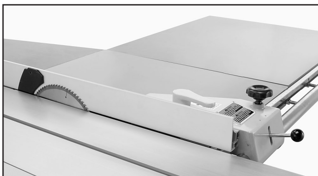
Figure 41. Fence against blade as a guide for aligning the scoring blade.
